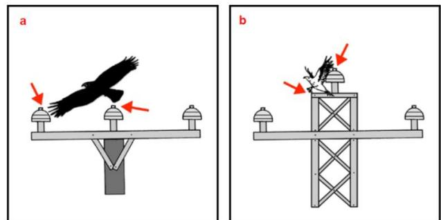
**Figure 21:** Electrocution occurs on certain supports on which birds can easily touch two conducting wires (a) or touch the pylon and one of the wires (b), thereby receiving a fatal electrical discharge. Modified from Janss & Ferrer (1999).
