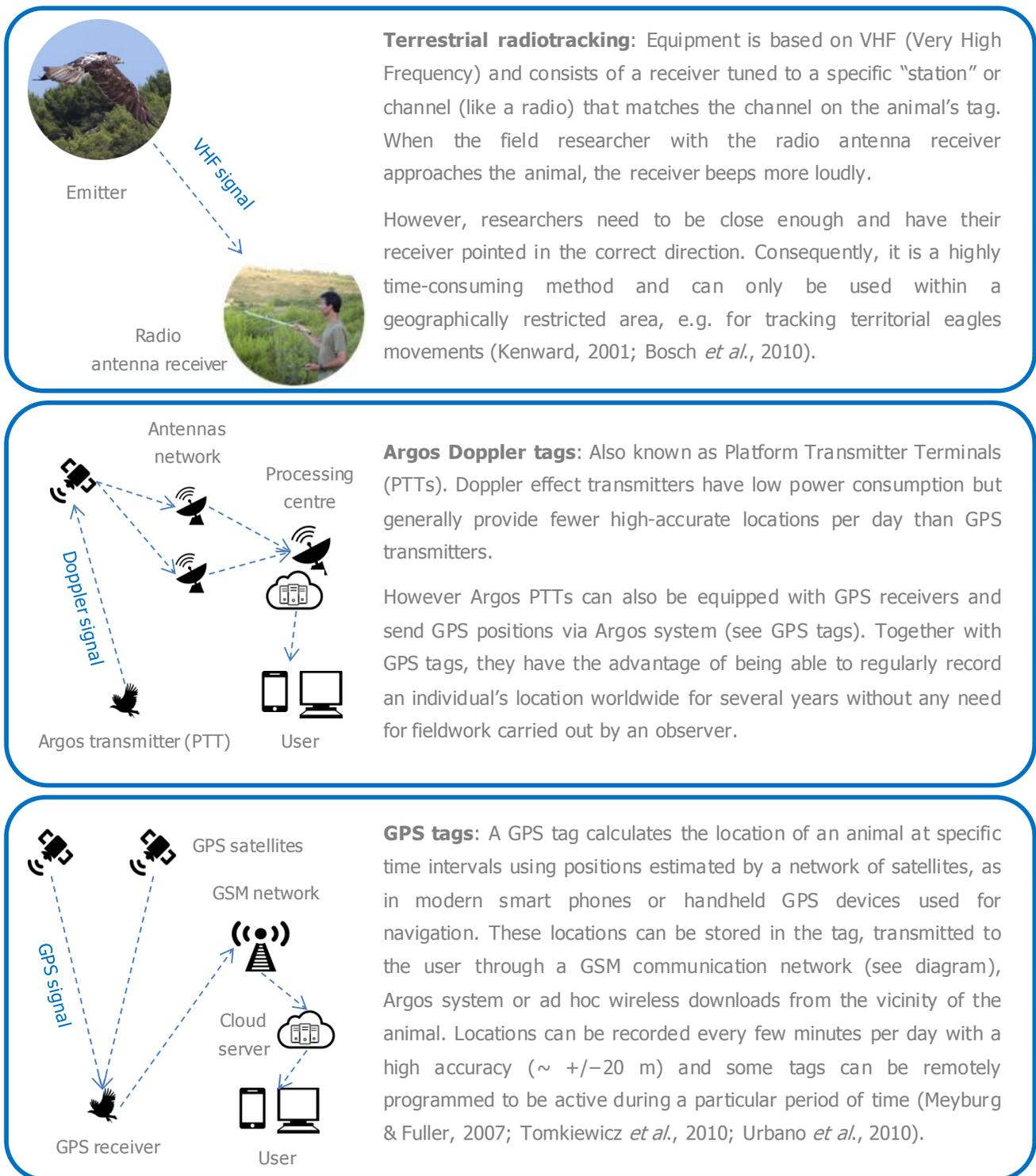
Figure 7: Characteristics of the main three broad systems for remote tracking wildlife movements and behaviour.
